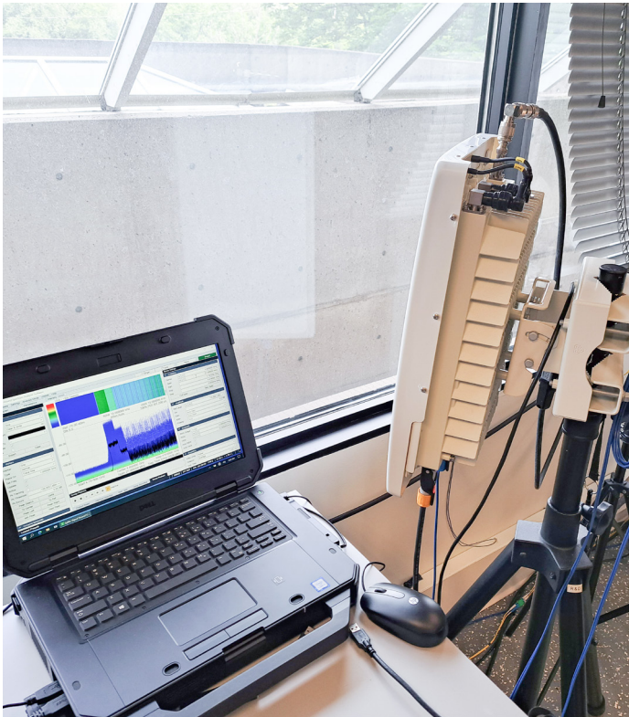
FRMCS under test in the lab, Toronto. ORAN AIO (All In One) small cells. The lab operates in 5G SA mode in band n77 and n79. Photos Thales.
